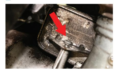
Remove bolts from hard lines in the top of cooler and bolts attaching cooler to transmission.
