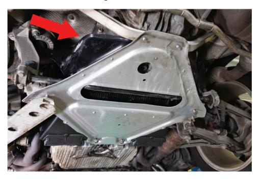
NOTE: The lower diamond brace does not need to be removed from the car for the install, but the plastic baffles will need to be trimmed to fit the cooler. In this application the rivets were drilled out and the baffles were removed entirely, but that is not necessary.
