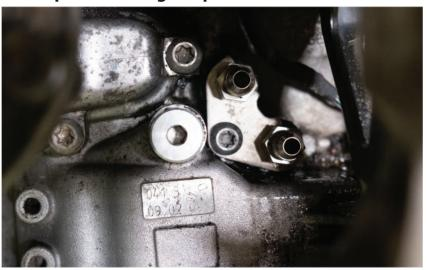
Loosen lower bolt and remove top bolt on transmission mount.
