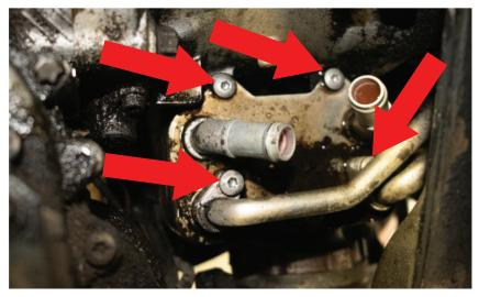
Access to bolts is easier through top of engine compartment. Remove cooler through bottom.
