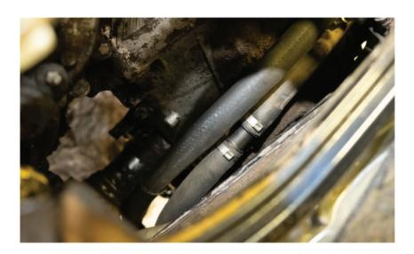
Insert PDK fittings into transmission and replace holding clasp.
