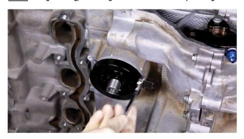
In the next steps, you will fit the IMS Solution oil feed hose to the Spin On Filter Adaptor, and the IMS Solution Flange. The completed hose assembly should appear like the photo below.
