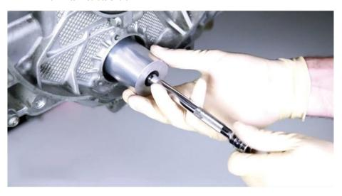
Place protective shim over IMS Solution bearing. With shim in place, install IMS bearing snap ring.
