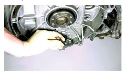
Using a 3mm (1/8 in) drill bit, drill a pilot hole in the crank case.
