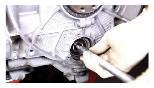
Slide puller body of threaded rod. Install puller washer and nut onto puller and lubricate.
