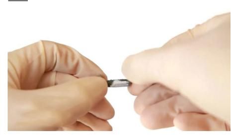
Once IMS Solution flange is flush with crankcase, install IMS Solution flange fasteners finger tight.
