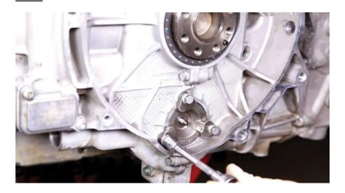
Using two flatblade screwdrivers, gently and evenly lever off the IMS bearing flange, then remove from engine.
