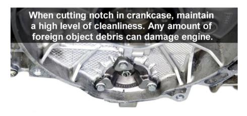
Using the IMS Solution flange as a guide, mark the center of the crank case using an awl.
