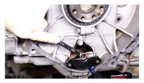
Once center stud nut has been a installed finger tight, torque IMS flange bolts.
