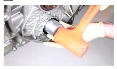
Once bearing is fully installed and bottomed out, remove the installation tool from intermediate shaft.
