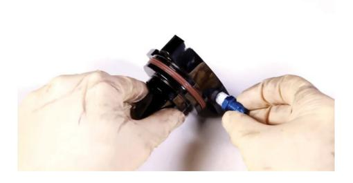
Using the provided assembly lube, lubricate bearing contact surface on IMS Solution flange.
