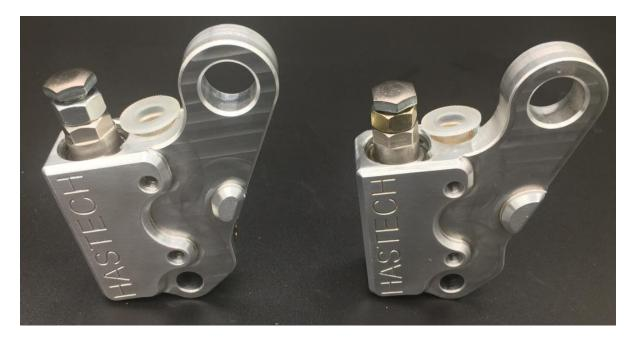
Remove the plastic 'hats' before installation, the tensioner is oil filled with regular engine oil and they are there to avoid spill during transport.
