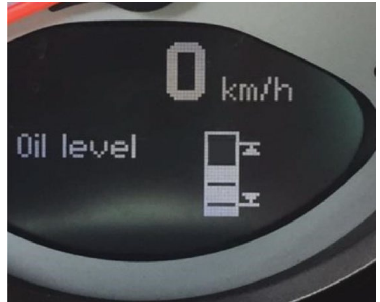
Electronic level indicator in the instrument cluster
