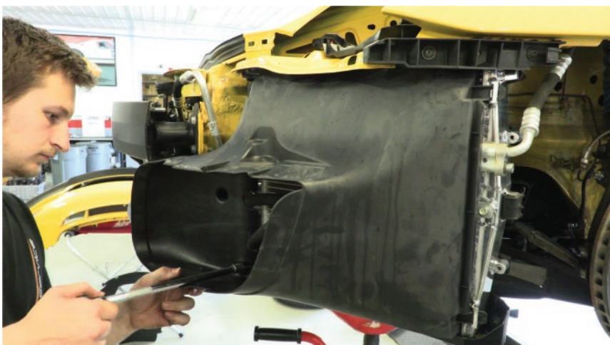
► Install radiator shroud. Working behind the shroud, align line clamps so that the shroud mounting bolts can be pushed through their holes. Insert and tighten the bolts to radiator.
